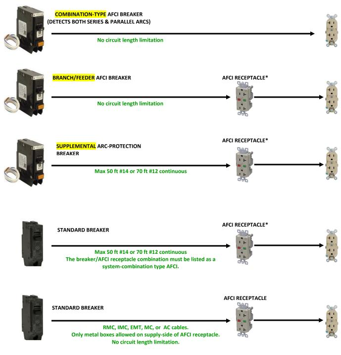
\*An outlet/branch circuit type AFCI unit used in this scenario is required to be marked as the first outlet of the circuit. Circuit breakers and devices must be listed. Always read and comply with applicable electrical codes. This page is a summary only. NEC is a registered trademark of the National Fire Protection Association.
